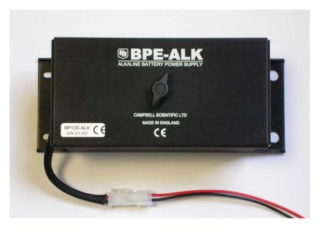
Before installing the alkaline batteries, connect all necessary sensor leads, control lines and power leads. The datalogger can be turned off and on by disconnecting and reconnecting the in-line connector between the BPE-ALK and the datalogger.
