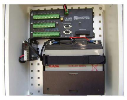
Figure 2(b) CH100 charger mounted alongside a BP17 in a typical loggerenclosure configuration
