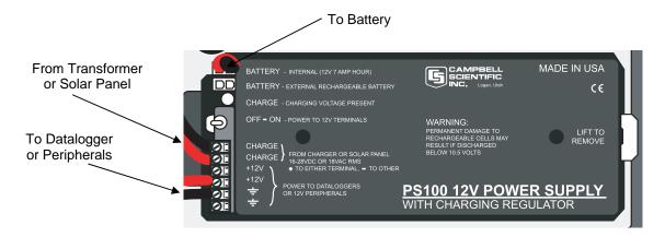
Figure 3. Wiring to Charger
