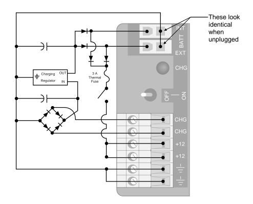
Figure 4. Simplified Charging Circuit Schematic
