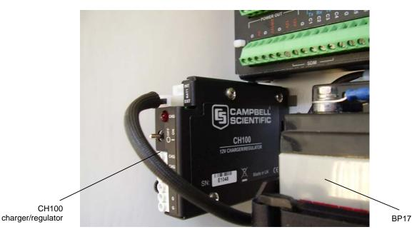
Figure 2(a) CH100 charger mounted alongside a BP17 in a typical loggerenclosure configuration
